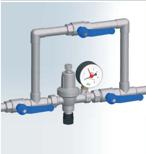
By-pass installation overview
