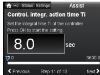
Fig. 44 Control. integr. action time T_i
