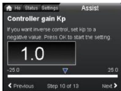
Fig. 43 Controller gain K_p
