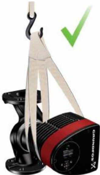
Fig. 10 Correct lifting of pump
