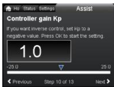
Рис. 43 Controller gain K_p
