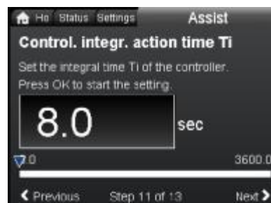
Рис. 44 Control. integr. action time T_i
